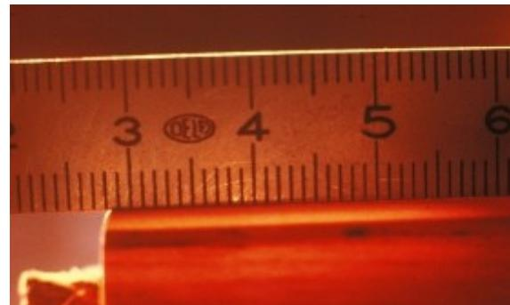
The top of the block must **never** be convex otherwise the air stream cannot be correctly focused. If this happens it should be corrected by filing or scraping as shown below.
