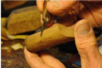
First remove a little wood from underneath, so that it can rest lower. This can be done by scraping with a knife or scraper, or by filing.
