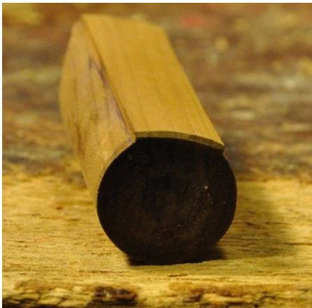
The top of the block is slightly concave lengthwise and, crosswise, it should have the same curvature as the labium. In some recorders it can be flat, if the windway and labium are made in this way. At the inside end there is a small chamfer, about 1 mm deep, which plays a very important part in stabilising the sound and the speech of the instrument. It must under no circumstance be modified without a valid reason. Any mistake here can be disastrous
