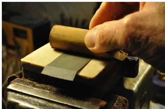
Place a strip of fine abrasive paper (320 grain), whose width is equal to half the length of the block or less, on a perfectly flat surface. Hold the block upside down and rub it lengthwise from one end to the other on the paper. The effect will be greater on the middle of the block than on the ends, and this will preserve its concave profile.
